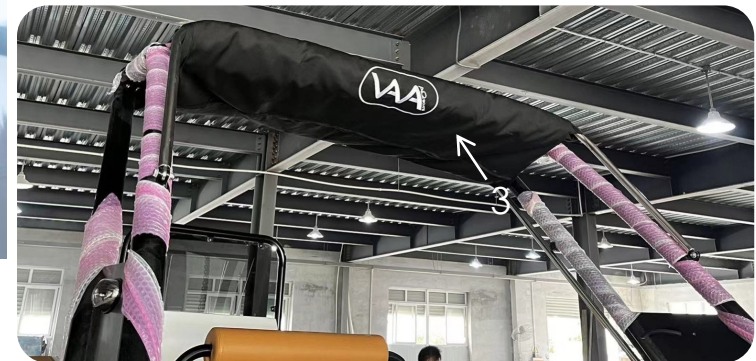
1. Navigation lights 2. Bimini stainless steel reinforcements 3. Bimini fabric case 4. Wake tower speakers
