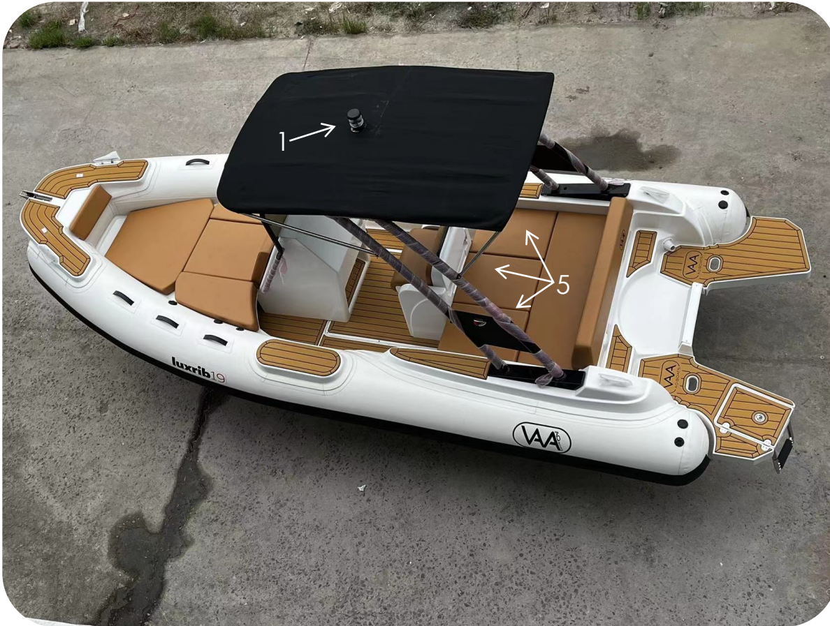
1. White light 360° 2. Navigation light 3. Bimini stainless steel reinforcements 4. Bimini fabric case 5. Removable cushion at the back*
